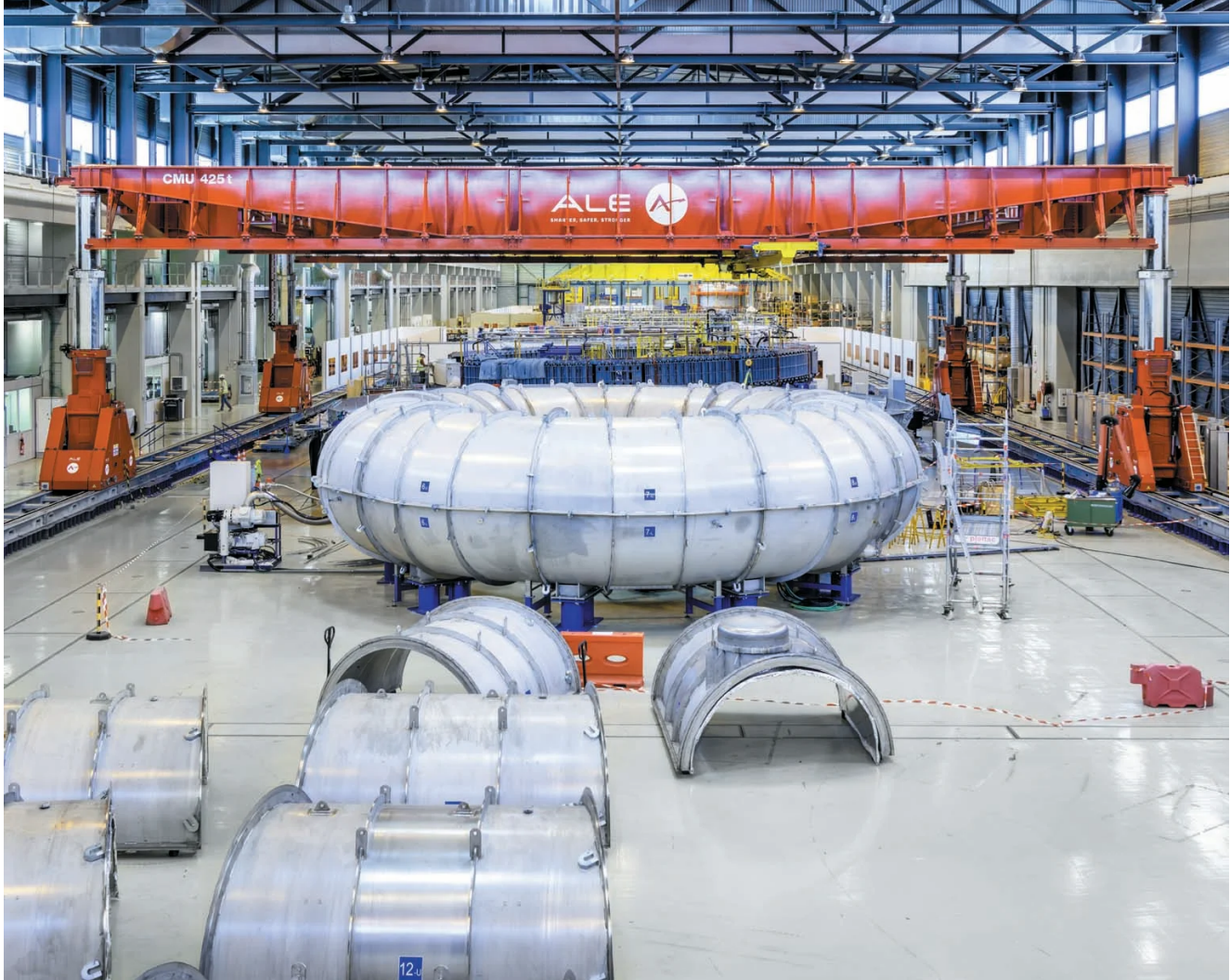
At the site of the International Thermonuclear Experimental Reactor (ITER), a poloidal field coil undergoes testing. Six of these ring-shaped magnets will steer plasma within the experiment. Credit: Alastair Philip Wiper
